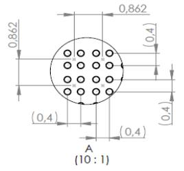
Material: Sharp edges to be chamfered!
