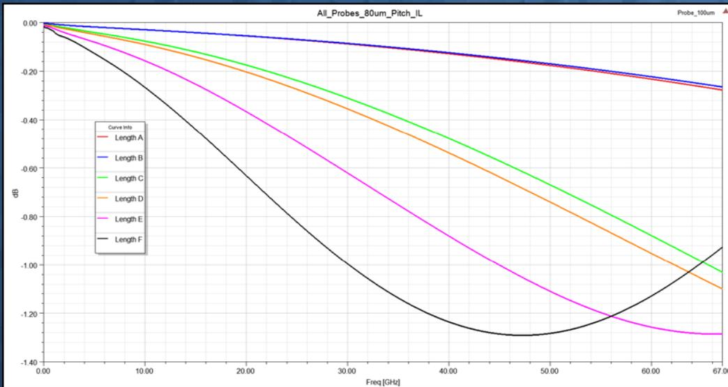
S21, Insertion Loss at 80 $\mu\text{m}$  pitch
