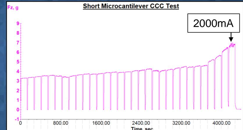
CCC Test showed no cantilever failure up to 2000mA
