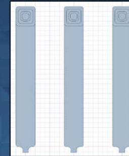
Microcantilever probes, top view
