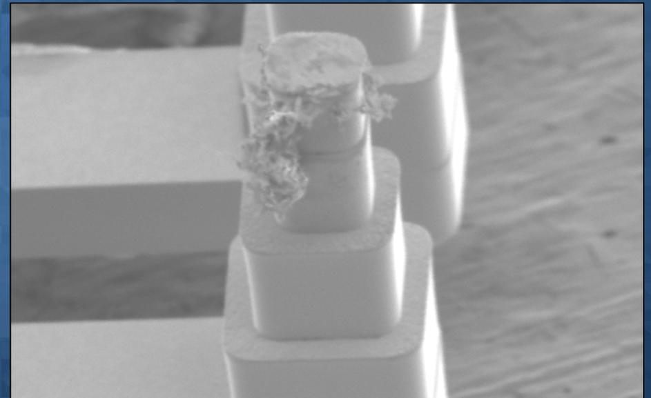
SEM image of a probe tip with foreign material.
