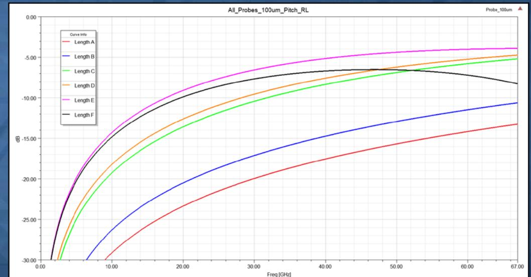
Return Loss at 100 $\mu\text{m}$  pitch
