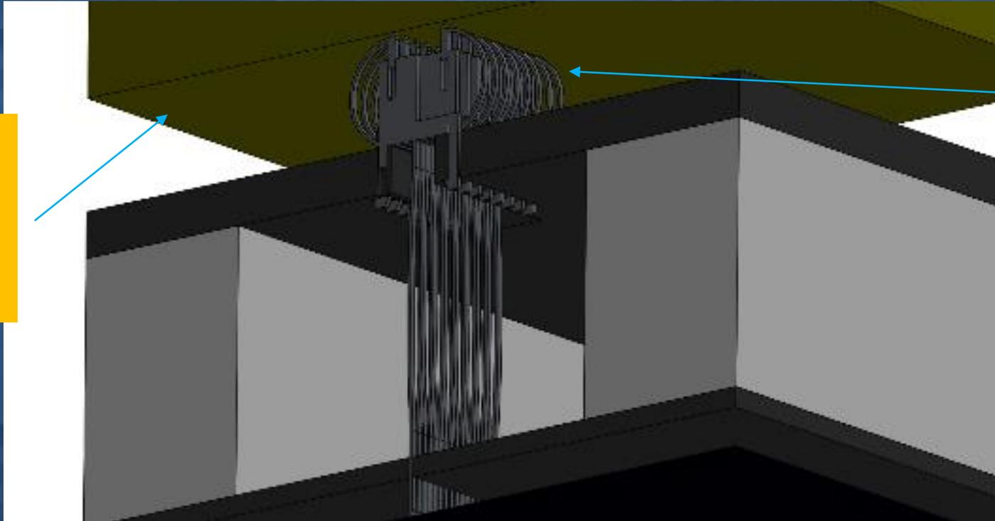
Distal side design MEMS probe allows for independent compliance to PCB
