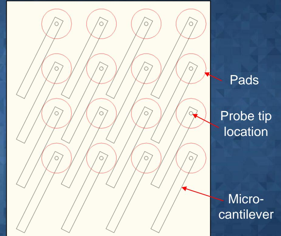
Microcantilever probe design for contacting 150 $\mu$ m pitch array
