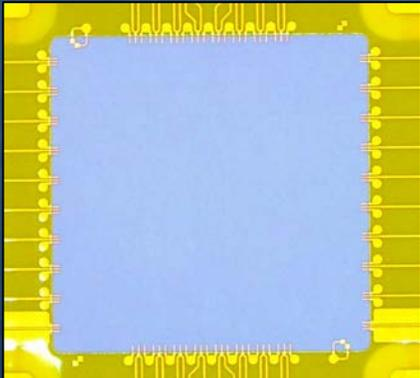
Microscope image of center design of FPC with pads
