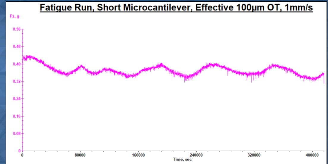
Fatigue run graph shows force over time at 14 cycles/second
