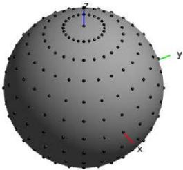
Constant Step Size Grid With  $\Delta\theta=\Delta\phi=15^\circ$  266 Points
