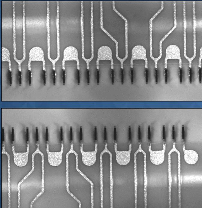
Microscope images of cantilever probes
