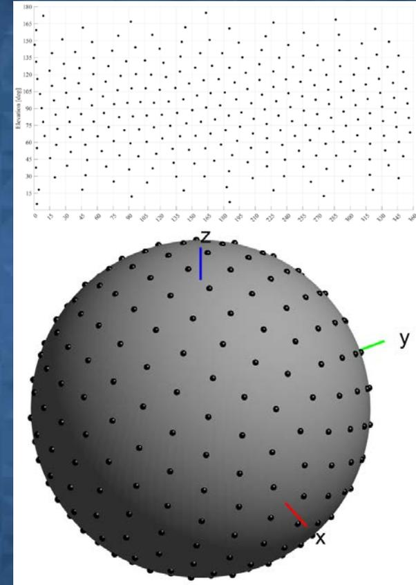
constant step size grid with  $\Delta\theta=\Delta\phi=15^\circ$  - 266 points
