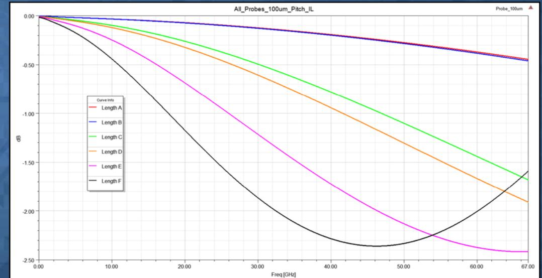
S21, Insertion Loss at 100 $\mu\text{m}$  pitch
