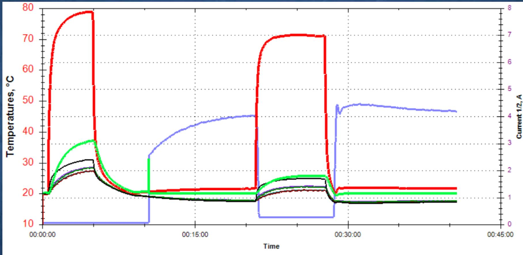
**K-value = Delta T / Power = 50K / 500 = 0,1 k/W -> Chip Temp = +70°C at +20°C Chuck**
