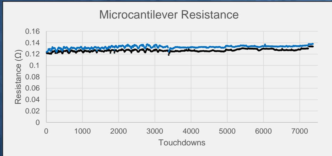
Resistance includes microcantilever probe and flex microstrip
