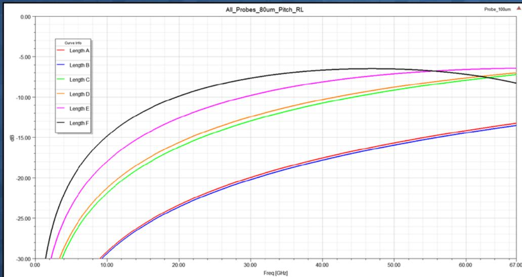
Return Loss at 80 $\mu\text{m}$  pitch
