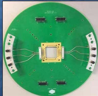
Tester side of PCB with 6 coaxial cables attached
