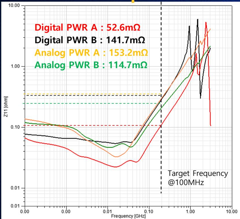
Impedance Deviation between DUTs [63DUT]
