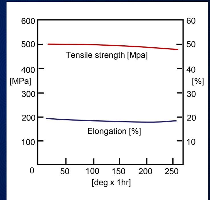
Characteristics of general sample Ni-e.f. material at high temperature
