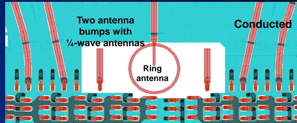
mm Wave Probe Connection: 2 to 1 combining with 1/4-wave antennas
