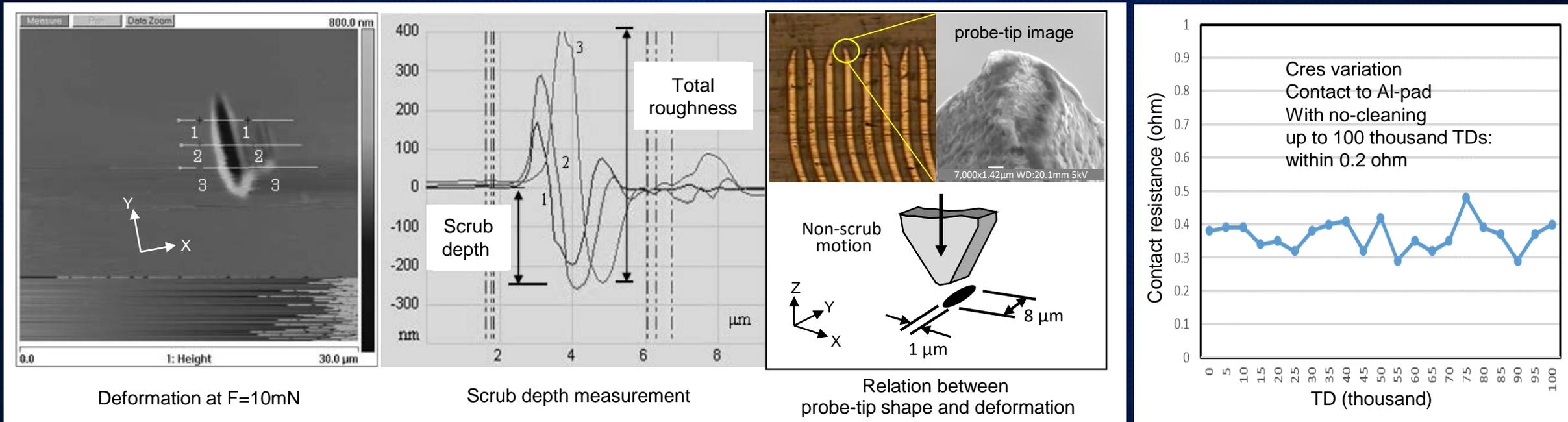
Probe mark of the non-scrub design probe at contact force of 10 mN
