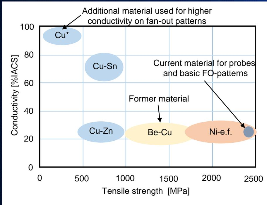
Relation between Tensile-strength and Conductivity
