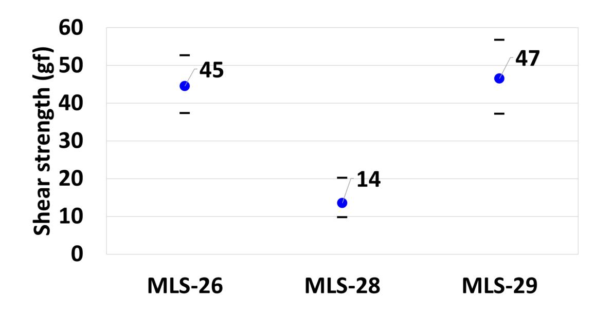
Shear strength of MLS-29 √Equivalent to MLS-26 √Three times higher than MLS-28
