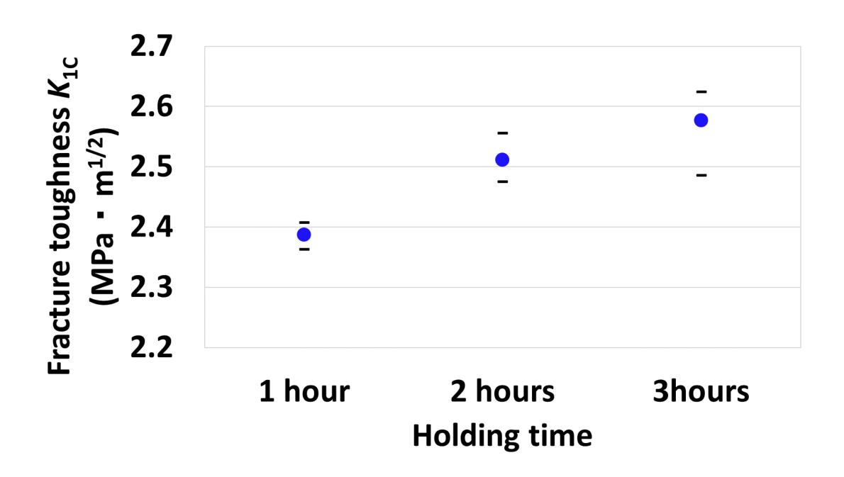
✓ Increasing the sintering time promotes crystallization in the glass region, leading to higher fracture toughness.
