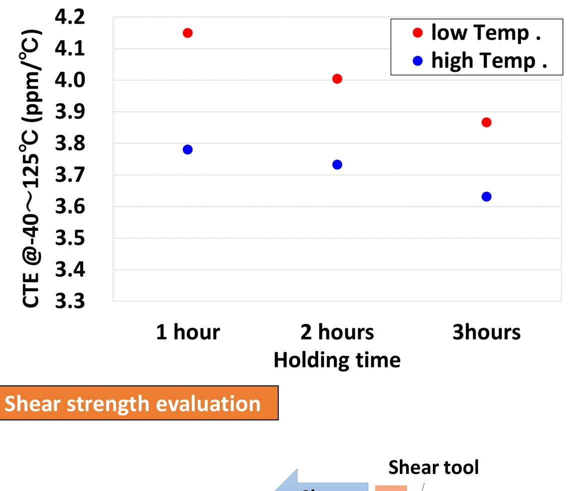
✓ The higher the sintering temperature, the lower the CTE.
