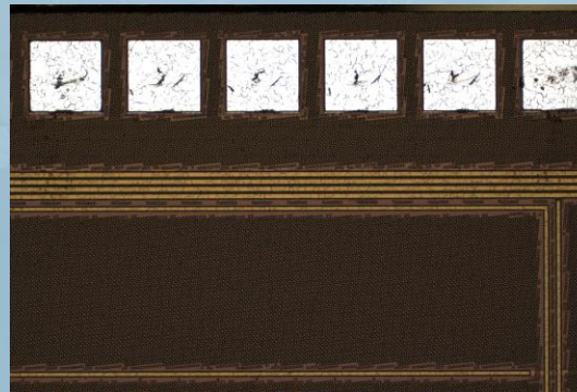
Scrub Mark after Testing RT \rightarrow mK \rightarrow RT
